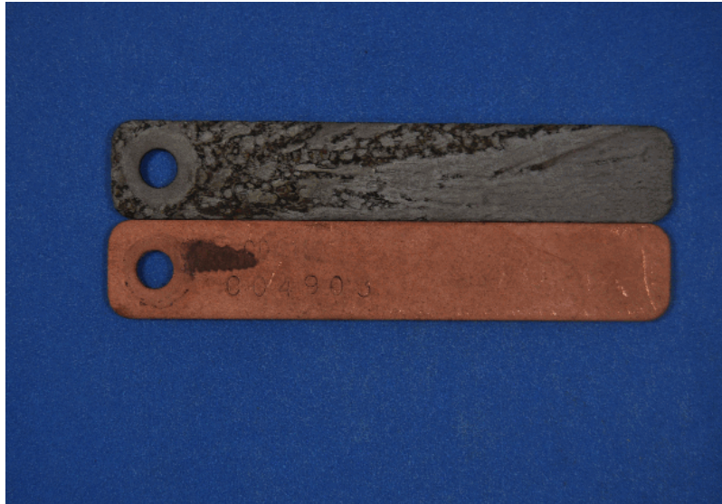
Photograph of actual coupons installed in system.
